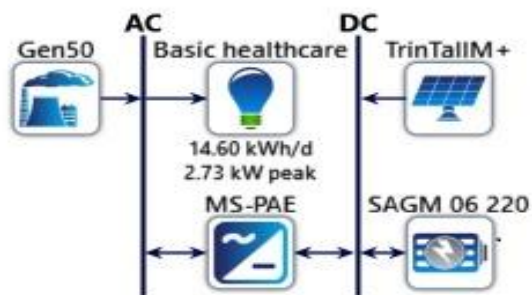
Fig. 3. The schematic diagram of the hybrid PV-diesel-battery energy supply system as arranged in HOMER pro modeling software.
